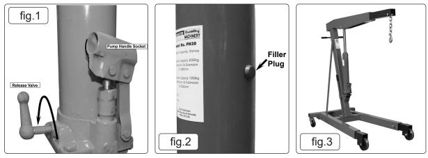
NOTE: The crane MUST be kept clean and dry and must be maintained in accordance with these instructions.
